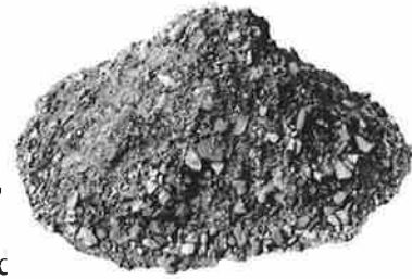
Fig. 6: A granular texture, usually with lumps, denotes a “Generally Granular” type of bulk solid.
